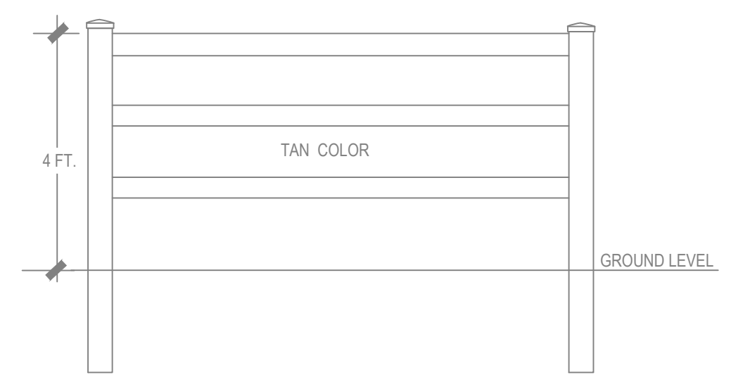
7 Vinyl 4' Open Rail Fence Detail L2 N.T.S.
