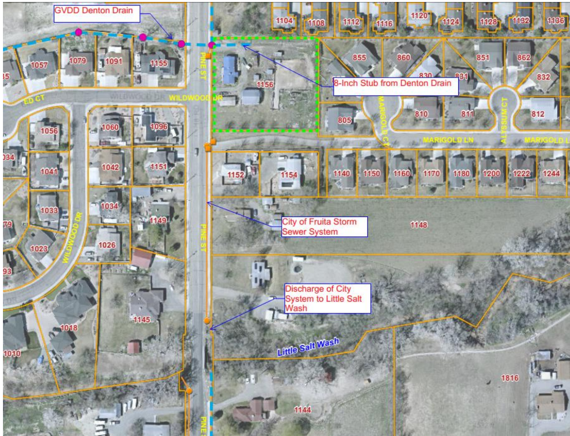
Existing Drainage Facilities
