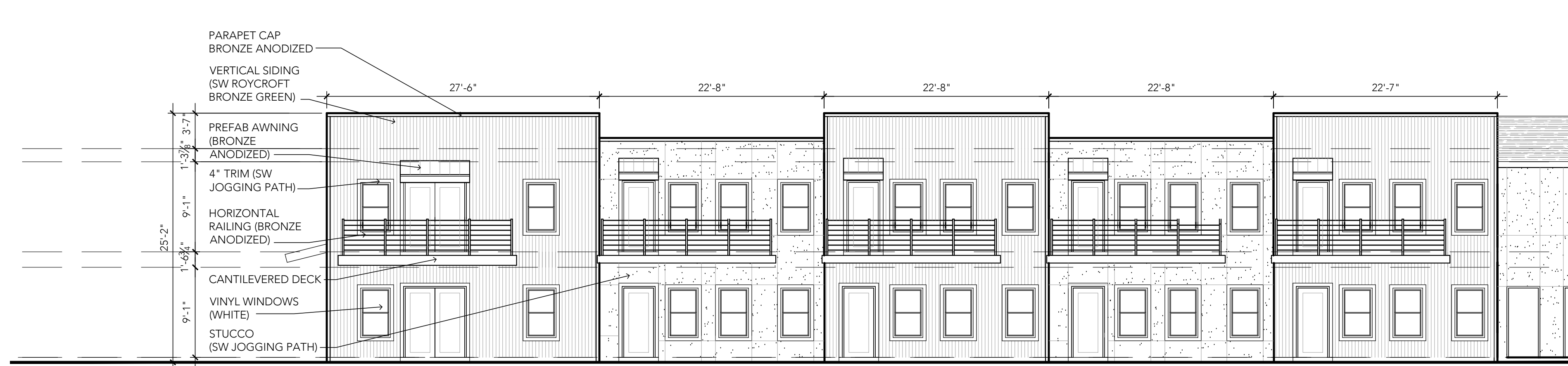
1 BUILDING 2 - NORTH ELEVATION 1/8"=1'-0"
