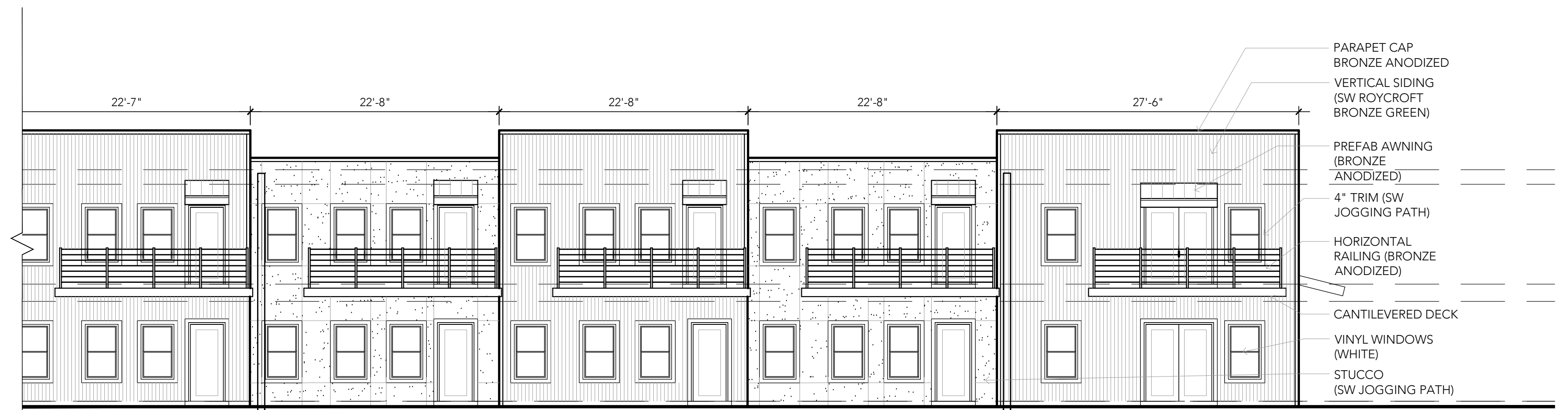
2 BUILDING 2 - SOUTH ELEVATION CONTINUATION 1/8\"/>
