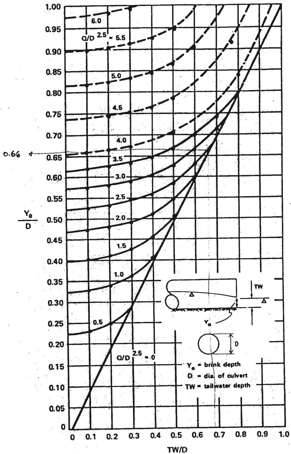
Applicable for  $TW < d_c$ . Enter  $TW/D$ , go vertical to  $Q/D^{2.5}$ , read horizontal to  $Y_o/D$ .
