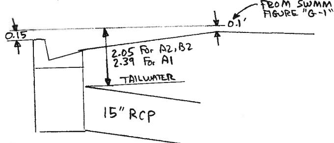
$$Q = CA \sqrt{2gh} \quad C = 0.8 \\ A = \left(\frac{\pi D^2}{4}\right)^2 \quad A = 1.23 \text{ ft}^2 \\ g = 32.2 \text{ ft/s}^2 \\ h = 2.05 \text{ FT}$$
